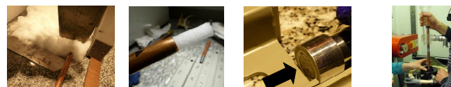
Sampling a cylindrical core into a snow slab Diameter = 1 cm Length = 1 cm Inserting into the aluminium sample holder Placing the sample holder into the cell
