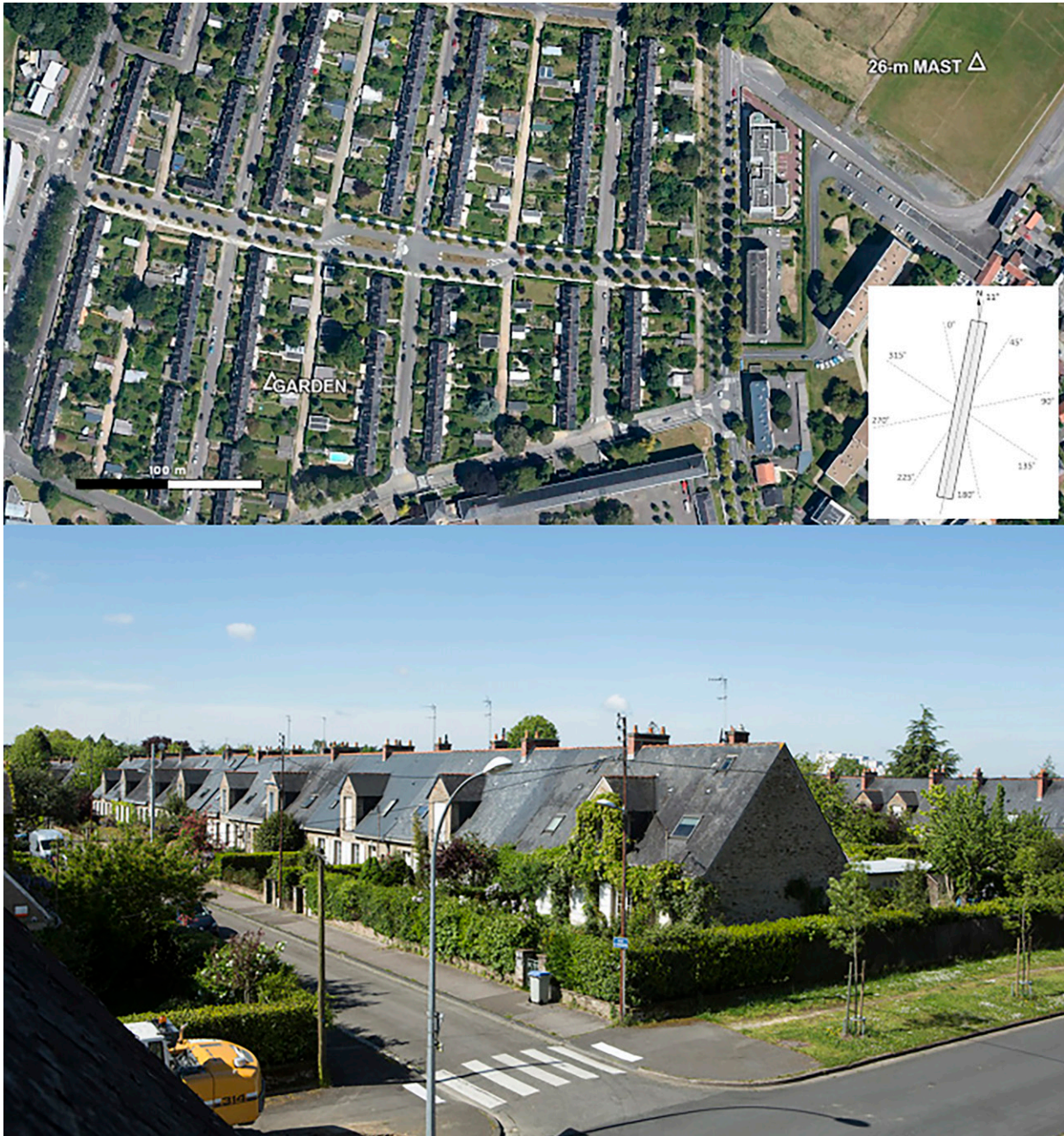
FIG. 1. Aerial photograph of the study site (source of map data: Google Maps) with location of the instrumented garden and of the 26-m flux measurement mast, and street picture of the neighborhood (source: copyright S. Marc). The inset diagram in the upper photograph describes how the 45° wind sectors are defined according to the mean orientation of the rows of houses.
