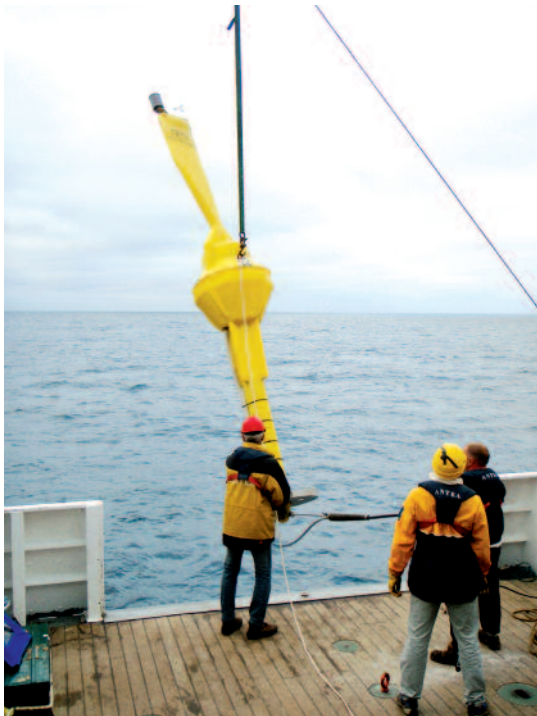
Deployment of Marisonde NG by RV Antea (Copyright Denis Dousse/Locean) for sea temperatures at depth during GOGASMOS in 2009 in the Bay of Biscay.
