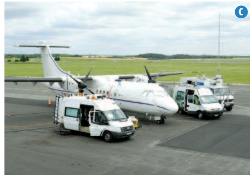
c - Intercalibration exercise with the ATR42 and the 3 instrumented vans.
