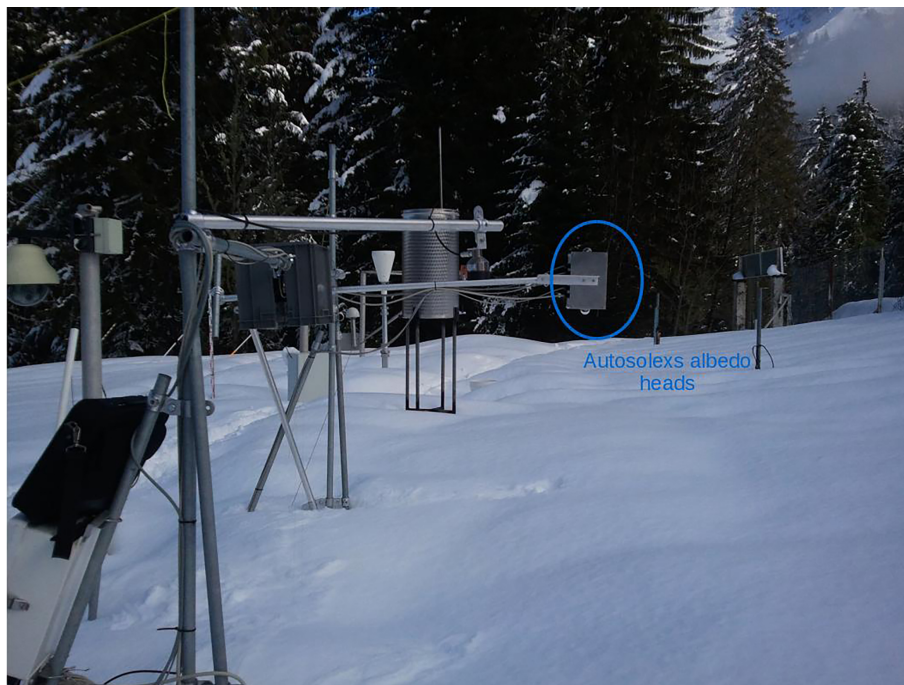
Figure 1. Part of the col de Porte field measurements site on 17 February 2014, 14:35. North direction is the left of the picture. The two measurement heads of Autosolex are circled in blue.
