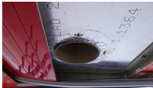
Figure 2. The rolling door at the bottom of the chimney through which FIRR takes measurements. The door is shown in optimal position for instrument stability, but nominal position is completely on the left. Flight direction is towards the left.
