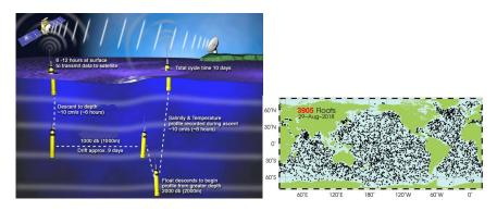
Figure 6 - a) Functioning of an ARGO float and b) the ARGO network on a given day (ARGO database).
