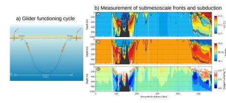
Figure 7 - a) Functioning of a glider and example of a b) potential temperature, c) salinity and d) oxygen concentration section across several fronts in the Mediterranean Sea (A. Bosse's PhD).
