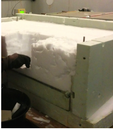
(a) Temperature gradient apparatus with side wall and upper plate removed to measure density gradient and SSA.
